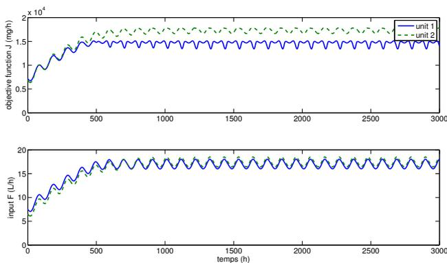
Fig. 4. Results of the multi-unit optimization method with simultaneous correctors applied to two non identical bioreactors
