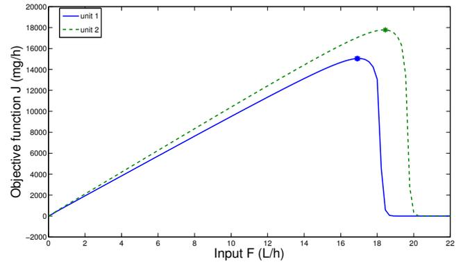
Fig. 3. Static characteristics of the two non identical bioreactors
