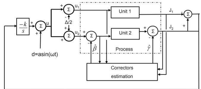
Fig. 2. Structure of the multi-unit optimization method with simultaneous adaptive correctors
