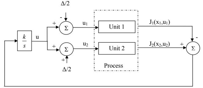
Fig. 1. Schematic for multi-unit optimization
