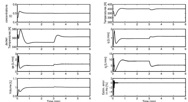
Fig. 2. Closed-loop nominal reactor behavior with ST observer based controllers with actuator filters.
