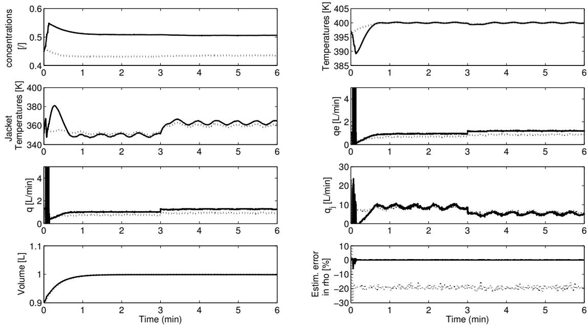
Fig. 3. Closed-loop robust reactor behavior with ST (cont. line) and EKF - observer based (dotted line) controllers without actuator filters.
