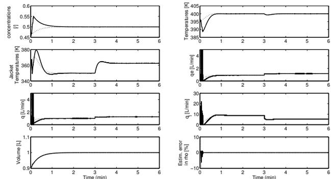
Fig. 1. Closed-loop nominal reactor behavior with ST (cont. line) and EKF - observer based (dotted line) controllers without actuator filters.
