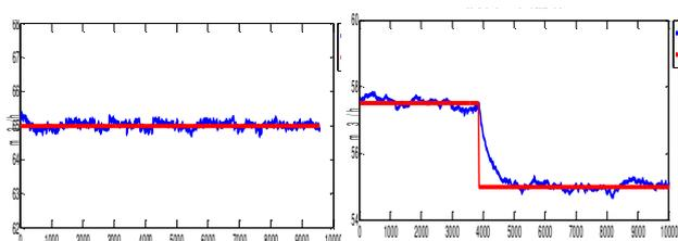
Fig. 10: Class C valves: PV and SP (red) trends
