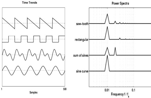
Fig. 1. Time trends and Periodograms of different signals toothed' or triangular signal produces both odd and even harmonics.
