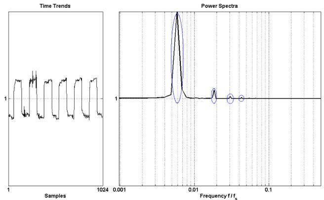
Fig. 3. Time trend (left) and power spectrum (right) of a control loop suffering from stiction
