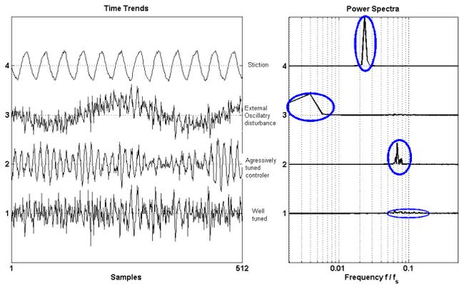
Fig. 4. Time trend and power spectra of controller error (1) well tuned controller (2) controller with excessive integral action (3) presence of external oscillatory disturbance (4) presence of stiction in the control valve.
