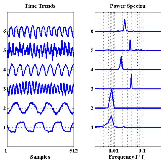
Fig. 5. Time trend and power spectrum of six different industrial data sets. (1) PC (2) FC (3) AC (4) LC (5) ThC (6) CC
