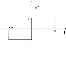
Fig. 2. Control signal in presence of Stiction
