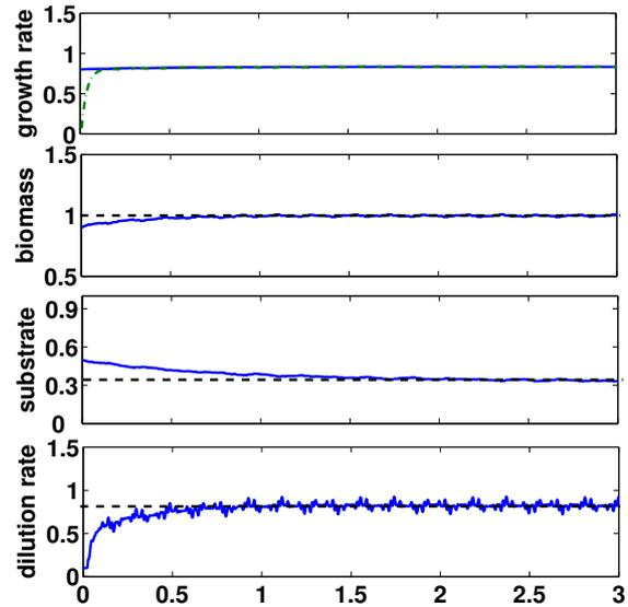
Fig. 4. Perturbed OF response for  $k = 3, \omega = 35$  and errors as given in the text. Solid line: OF response, dash-dotted line: reaction rate estimate, dashed line: set point value
