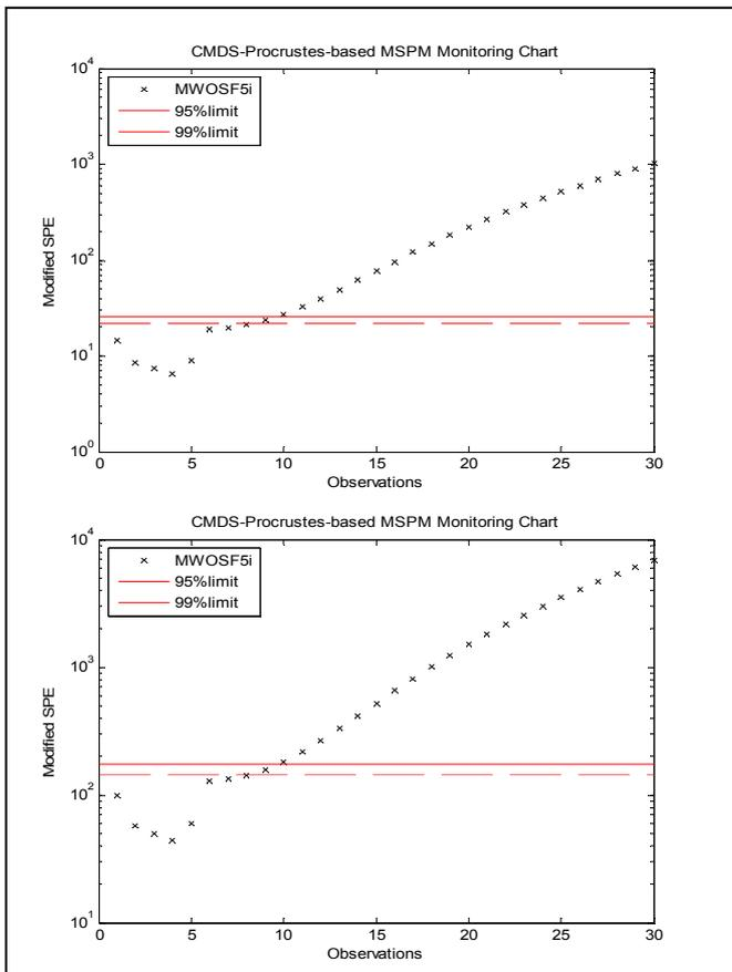
Fig. 4: FDI ( $C_r$ ) monitoring chart of CMDS-PA for incipient fault number 5 based on Euclidean scale (top) and city block scale (below)
