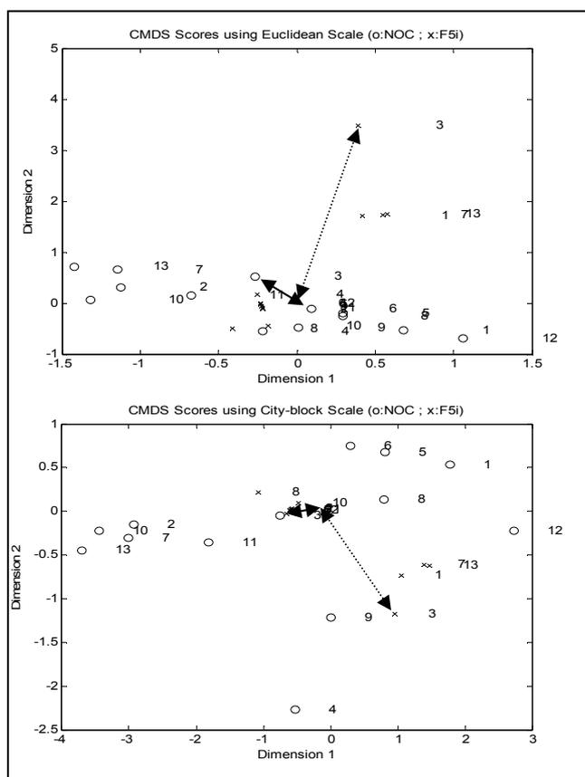
Fig. 6: Configuration plots of CMDS-PA for incipient fault number 5 between sample 1 and sample 12 based on Euclidean scale (top) and city block scale (below)
