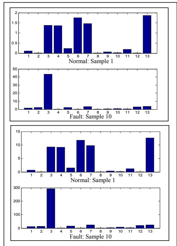
Fig. 5: Contribution plots of CMDS-PA for incipient fault number 5 based on Euclidean scale (top) and city block scale (below)
