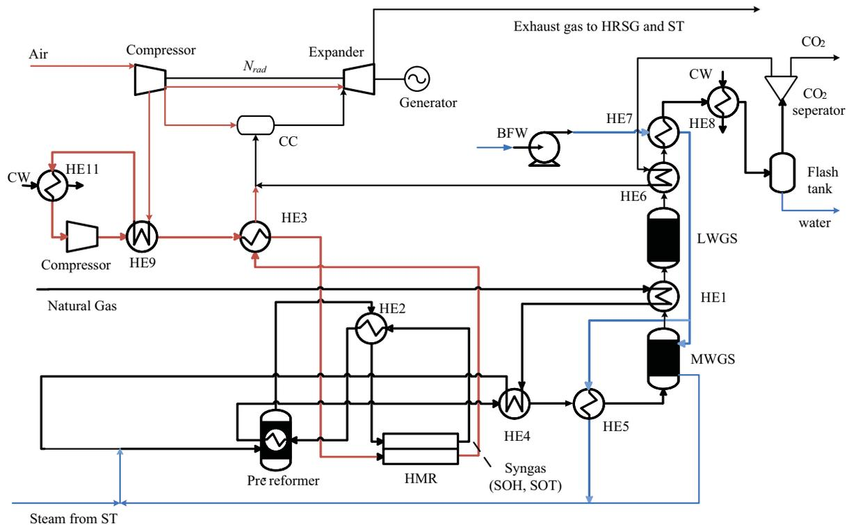
Fig 1. Sketch of the HMR process with HMR syngas reactor, CO<sub>2</sub> removal unit and gas turbine (Smith et al., 2009).
