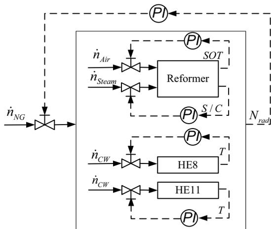
Fig. 2. Control structure for HMR power cycle.
