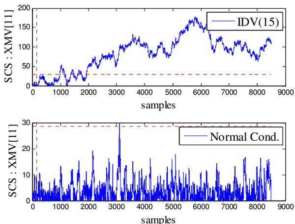
Fig. 4. The SCS for IDV (15); horizontal and vertical lines represent the statistical limit and the fault onset, respectively.
