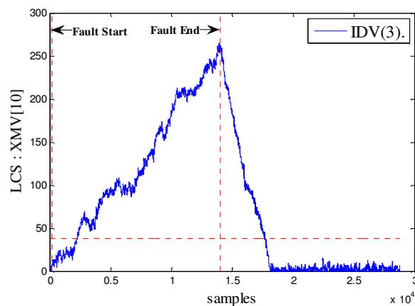
Fig. 3. The LCS for IDV (3); horizontal line represent the statistical limit. The vertical lines represent the onset (after 8 hours) and the end of the fault (after 700 hours).
