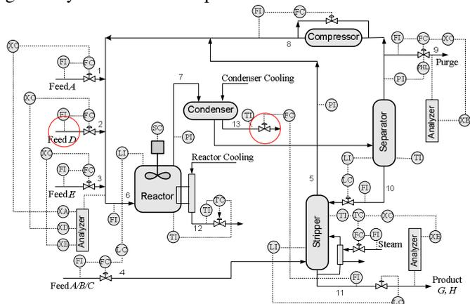
Fig. 1. Tennessee Eastman process with the second control scheme described in (Lyman and Georgakis, 1995); the circles indicate the location of the faults described in Table 1
