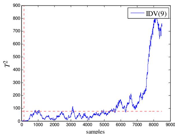
Fig. 6. The Hotelling'  $T^2$  for IDV (9); horizontal and vertical lines represent the statistical limit and the fault onset, respectively.
