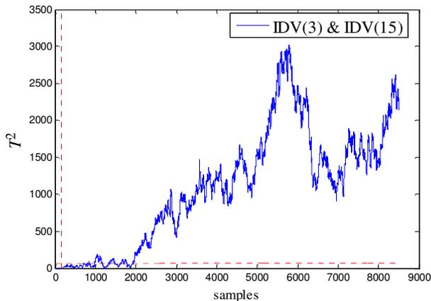
Fig. 7. The Hotelling's  $T^2$  for the simultaneous occurrence of IDV(3) and IDV(15); horizontal and vertical lines represent the statistical limit and the fault onset, respectively.
