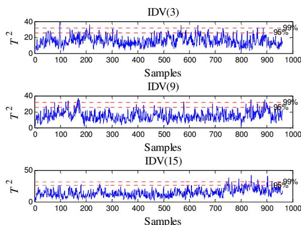
Fig. 2.  $T^2$  based on DPCA for the three unobservable faults of TEP, i.e. IDV (3), IDV (9) and IDV (15). The horizontal dotted lines represent the 95% and 99% confidence limits.
