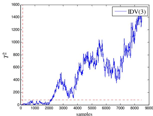
Fig. 5. The Hotelling'  $T^2$  for IDV (3); horizontal and vertical lines represent the statistical limit and the fault onset, respectively.
