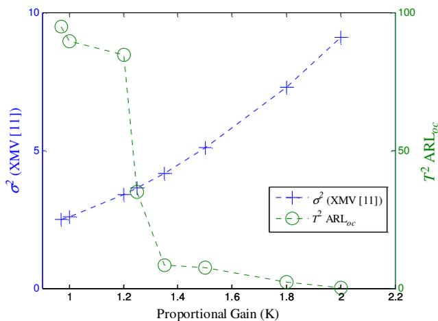
Fig. 8. The change in variability and the  $T^2$ - $ARL_{o.c.}$  as a function of the master controller's gain (XMV[11] is considered in the case).
