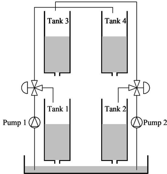
Fig. 1. Schematic diagram of the quadruple-tank process.
