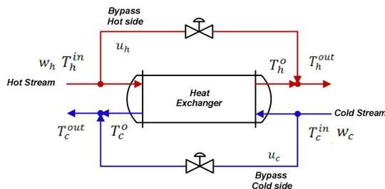
Fig. 1. General structure of a heat exchanger with bypasses.
