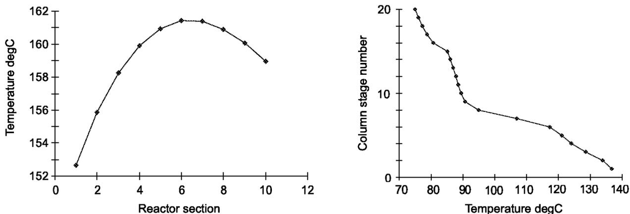
Fig. 3. Temperature profiles in the reactor (left) and the distillation column (right).
