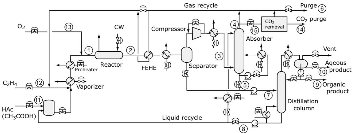
Fig. 1. Process flow diagram of the vinyl acetate monomer production plant. The stream numbers are the same as those of the original paper (Luyben and Tyreus, 1998).
