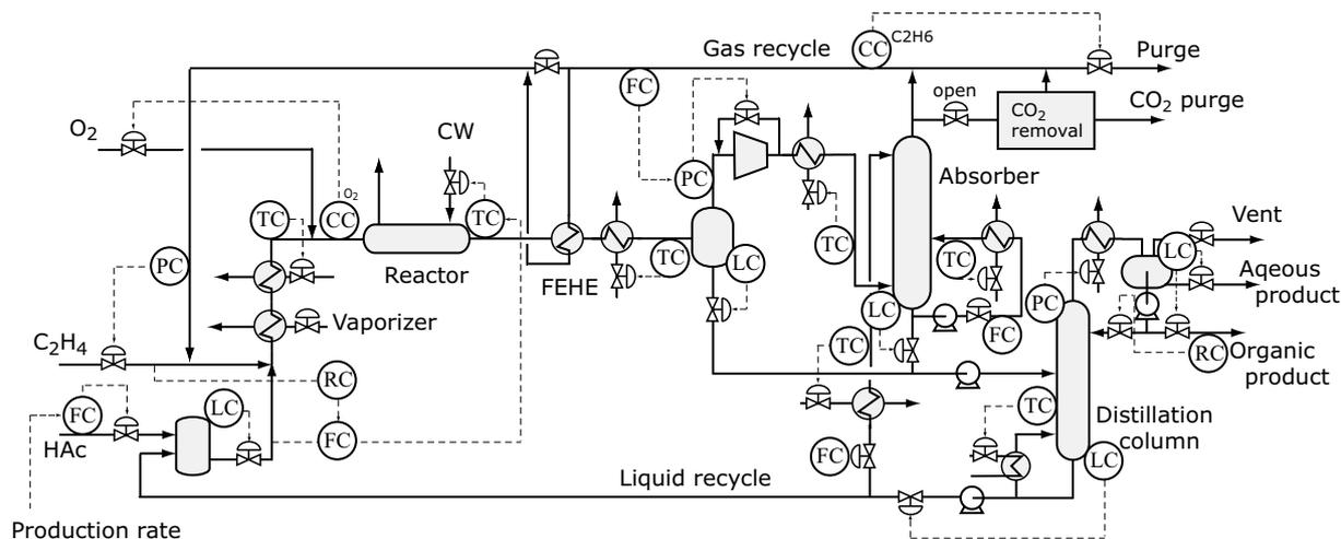
Fig. 4. An alternative control loop configuration. The fresh acetic acid feed is on flow control to set the production rate. A cascade loop from the liquid reactor feed flow to the reactor temperature setpoint is incorporated to ensure regulation of the acetic acid inventory.
