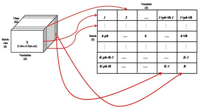
Fig. 2. Observation-wise with time-lag unfolding approach
