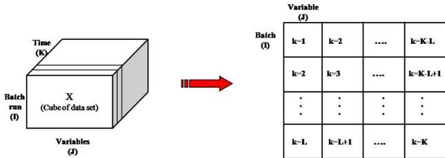
Fig. 3. Regularized Batch-wise unfolding approach
