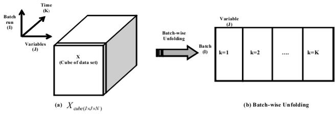
Fig. 1. Batch process dataset and batch-wise unfolding
