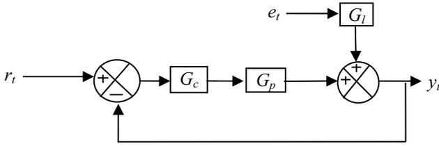
Figure 1: Generic Closed-loop Process
