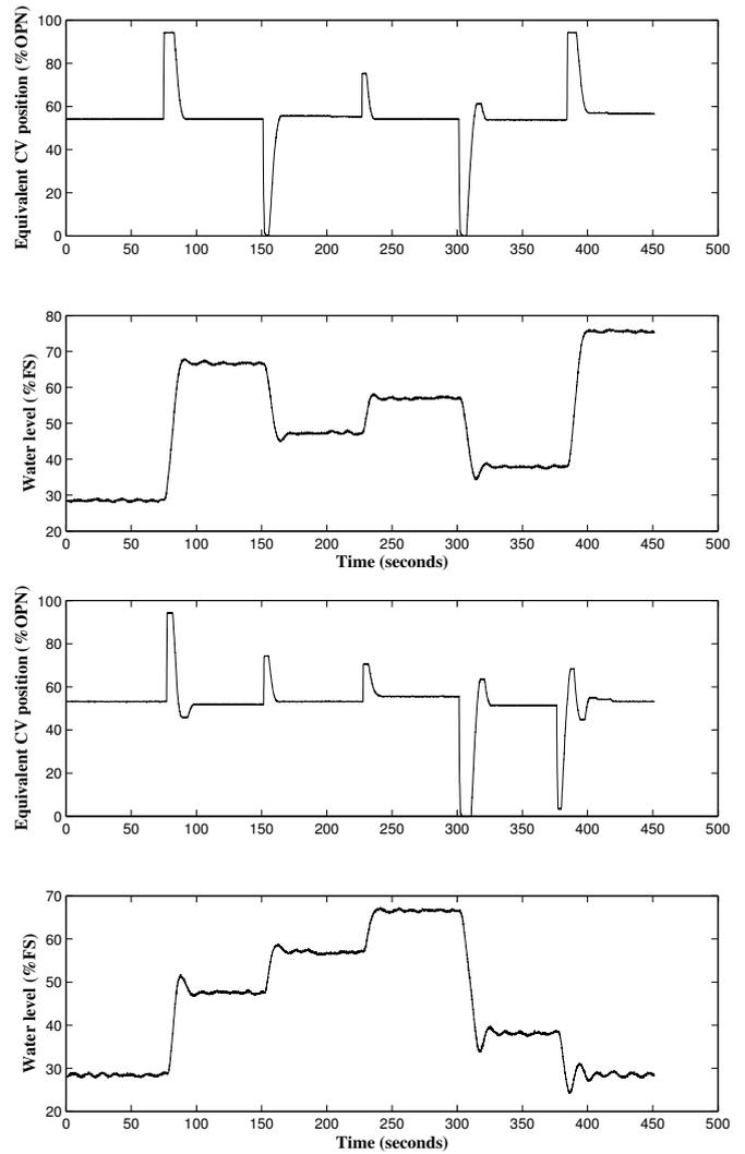
Fig. 1. (a) Input-output profile for training (b) Input-output profile for validation
