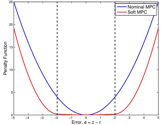
Fig. 4. Penalty function for Soft MPC and Normal MPC.
