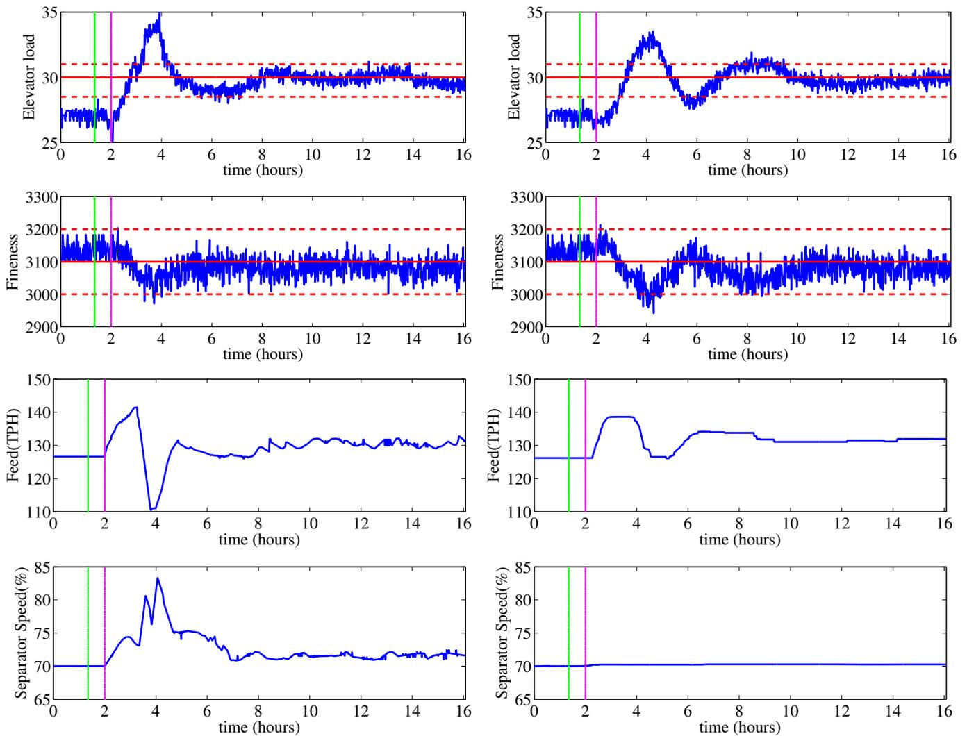
Fig. 5. Normal MPC (left) and Soft MPC (right) applied to a rigorous nonlinear cement mill simulator, ECS/CEMulator. The disturbances (change in hardness of the cement clinker) are introduced at time 1.35 hour (green line) and the controllers are switched on at time 2 hour (purple line). The soft constraints are indicated by the dashed lines.
