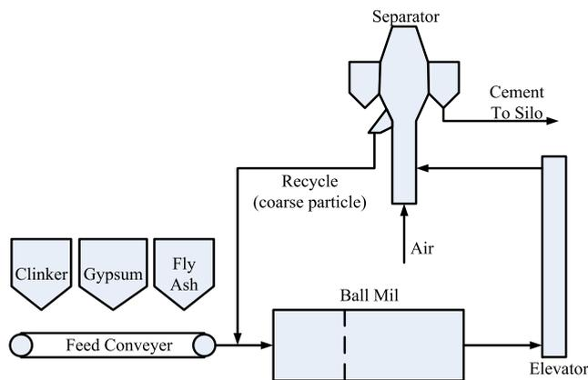
Fig. 2. Cement mill circuit.
