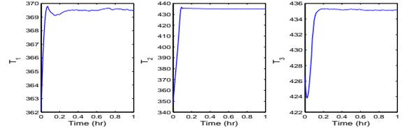
Fig. 3. Temperature trajectories of the process under the proposed DMPC design.
