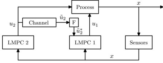
Fig. 1. Distributed LMPC control architecture (F means solving a feasibility problem).
