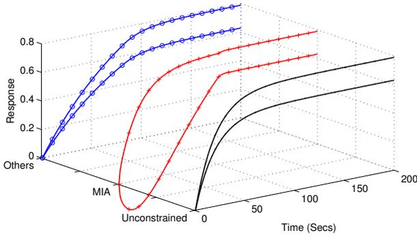
Fig. 6. Example 1: The Modified IMC (MIA, '+' ) yields a faster reponse for the first output at the expense of a poor transient response in the second out while the other schemes ( DP, OCT, ODC, OSS and two-stage IMC, 'o' ) all yield same response.
