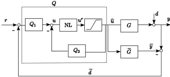
Fig. 4. The Modified IMC Structure with Directionality Compensation
