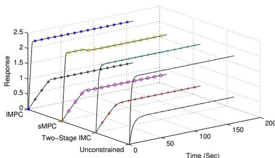
Fig. 8. Two-stage IMC (+) outperforms the single horizon MPC (sMPC, 'o') and yields similar response to long horizon MPC (IMPC, '\*')
