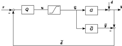
Fig. 2. The Conventional IMC Antiwindup Structure
