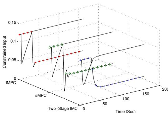
Fig. 9. Constrained input: Two-stage IMC (+), single horizon MPC (sMPC, 'o') and long horizon MPC (IMPC, '\*')
