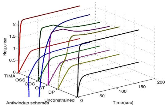
Fig. 7. Example 2: Two-stage IMC (TIMA) yields the closest performance to the unconstrained case. DP and OSS schemes have improved steady state behaviours but poor transient characteristics as opposed to the OCT and ODC schemes both of which have optimal transient behaviours but degraded steady state performances.
