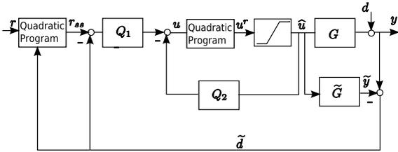
Fig. 5. The two-stage IMC Antiwindup
