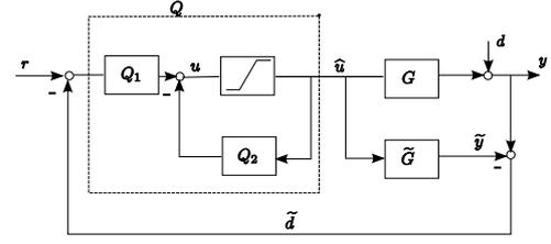
Fig. 3. The Modified IMC Antiwindup Structure
