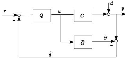
Fig. 1. The Standard IMC Structure
