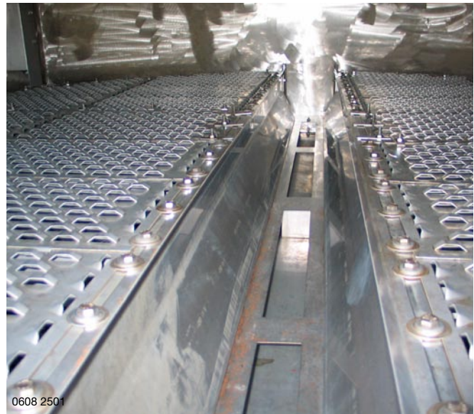
2-pass VG AF equipped with sloped outlet weir
