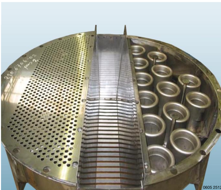
2-pass ConSep tray tested at FRI
