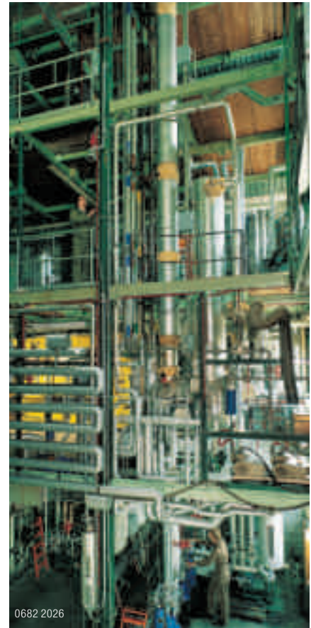
0682 2026 Multi-purpose pilot plant for the separation of mixtures by distillation, using Sulzer structured packings of various design
