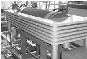
figure 1: 100l dyeing machine using carbon dioxide as a solvent.
