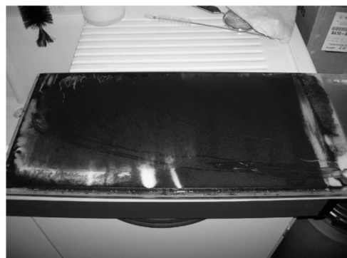
Biofilm of Chlorella on a polycarbonate plate
