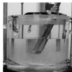
Fig.1: ATR FTIR, FT NIR sensors in crystallizer
