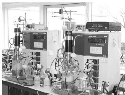
Fermentor setup used for P. pastoris cell cultures
