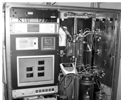
Figure 1: The equilibrium cell for CO 2 solubilities and induction periods determination: thermostated glass reactor, IR CO 2 gas detector, pH electrode, conductivity probe, temperature and pressure indicators, mass flow controllers.
