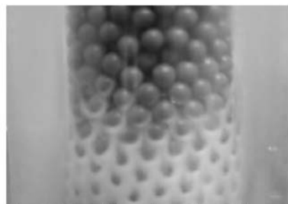
Fig. 1 – CO 2 desublimated onto the packing surface
