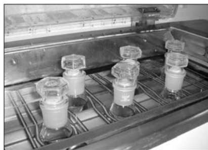
Figure 1: Batch experiments in shaking bath at fixed temperature
