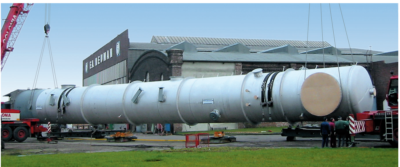
▼ Dividing wall column DN 3600
