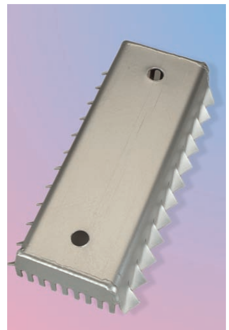
▲ Thormann® caps with the characteristic vapour slots for a controlled vapour flow into the liquid.
