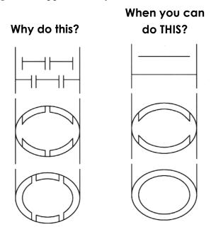
support structure requires time and money because all of the ring and bar pieces need to be engineered, fabricated, installed and welded.
