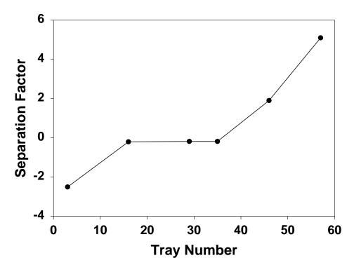
Figure 4 Separation Factor vs Tray Number From Bottom Showing Ineffectiveness of Middle 20 Trays (Pinch)
