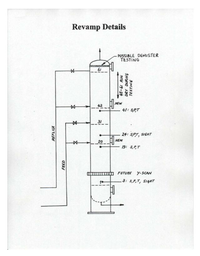
Figure 5 Detail of Column Revamp Showing Alternate Feed and Reflux Points, Positions of Sample Points (S), Pressure (P) and Temperature (T) Taps, Sight Glass Locations, and Position of Future One-Tray Detailed Gamma Scan
