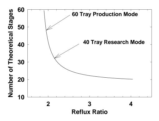
Figure 3 Number of Theoretical Stages vs Reflux Ratio for 4P Depropanizer Column
