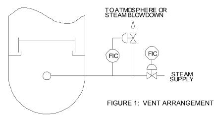
A steam sparger is used to introduce the steam into the tower. The pressure of the steam is monitored on the outside of the column, downstream of the flow control valve. When a slug
