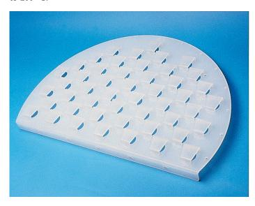
The key to the PROVALVE tray is its proprietary fixed-valve design with a uniquely tapered cover. The cover provides a forward-lateral push to the liquid across the tray, which improves liquid distribution and protects the tray deck from fouling.
