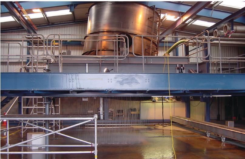
Testing of Model 961 enclosed channel distributor in the Koch-Glitsch test facility simulating wave motion.
