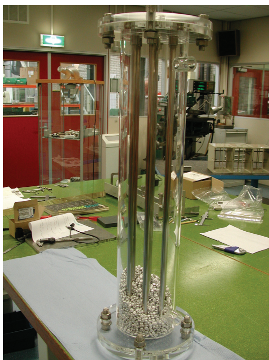
Show model of a membrane reactor for hydrogen separation during steam reforming.
