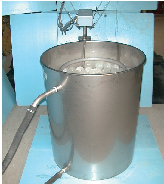
Test installation for testing phase change materials
