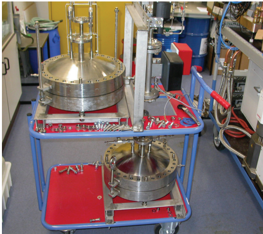
Test installation of a thermochemical heat pump
