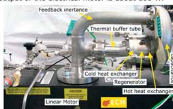
Lab-scale setup of thermoacoustic heat pump.
