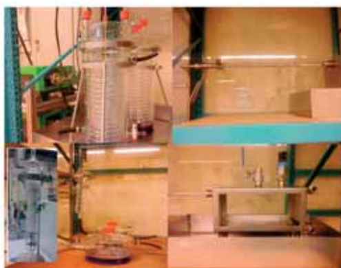
Constructed Static-mixer settler experimental setup for investigation of entrainment and droplet coalescence
