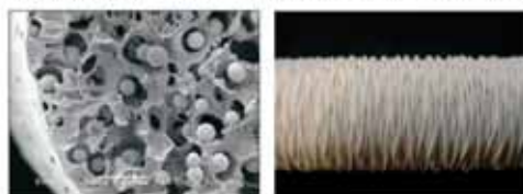
Combination of FILTRATION and ADSORPTION: MIXED MATRIX MEMBRANE fibers to form high capacity SEPARATION DEVICES.
