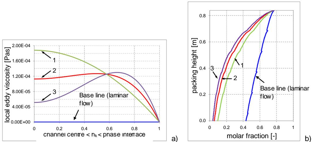
**Figure 8.** Influence of the eddy viscosity distribution on the concentration profiles in a packing bed: a) radial eddy viscosity distribution, b) calculated concentration profiles of a light boiling component
