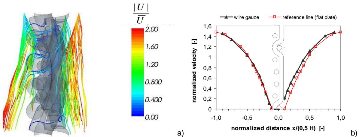
**Figure 3.** a) Streamlines around the wire; colour scale for velocity magnitude, normalised with its mean value; b) Calculated averaged velocity profile, H-distance between the layers
