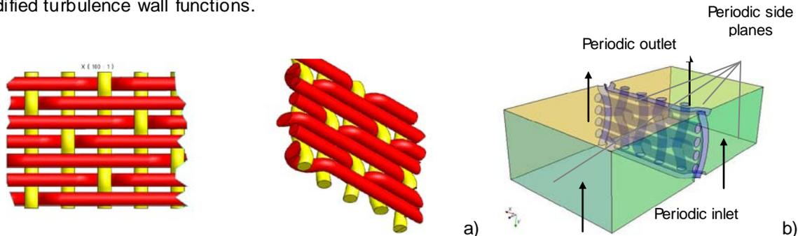
**Figure 2.** a) Structure of five-heddle-twill-weave wire gauze, b) periodic element used in the simulations
