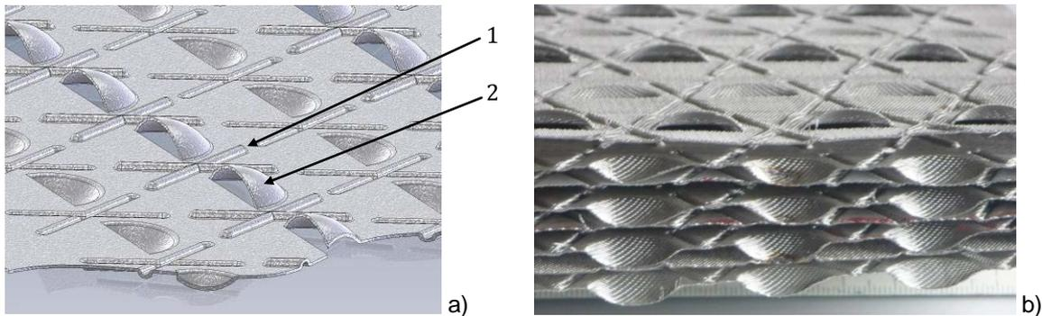
**Figure 1.** a) Single layer of the packing demonstrating the basic macro-geometry (patent pending): 1 – embossed formations to improve the packing performance, 2 – deep drawn spacers; b) Photograph of the packing
