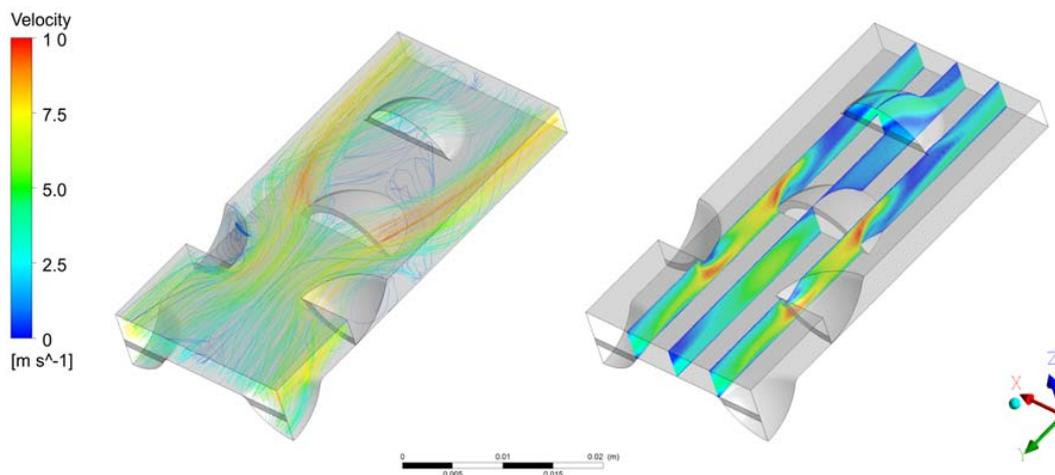
**Figure 5.** Streamlines inside the periodic element
