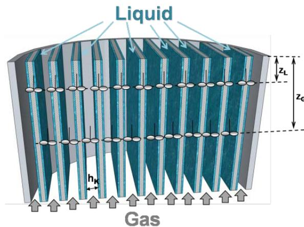
**Figure 7.** Hydrodynamic-analogy-based physical model of the investigated structured packing
