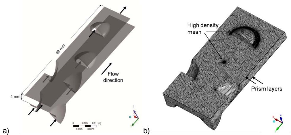
**Figure 4.** a) Periodic element of the packing, b) Computational domain
