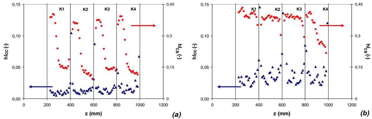
**Figure 4.** Axial distribution of liquid hold-up inside ( $hl_{CB}$ ) and outside ( $hl_{OC}$ ) the catalytic baskets of Katapak-SP11 obtained from measurements at liquid loads of  $4.62 \text{ m}^3/\text{m}^2/\text{h}$  (a) and  $23.1 \text{ m}^3/\text{m}^2/\text{h}$  (b)
