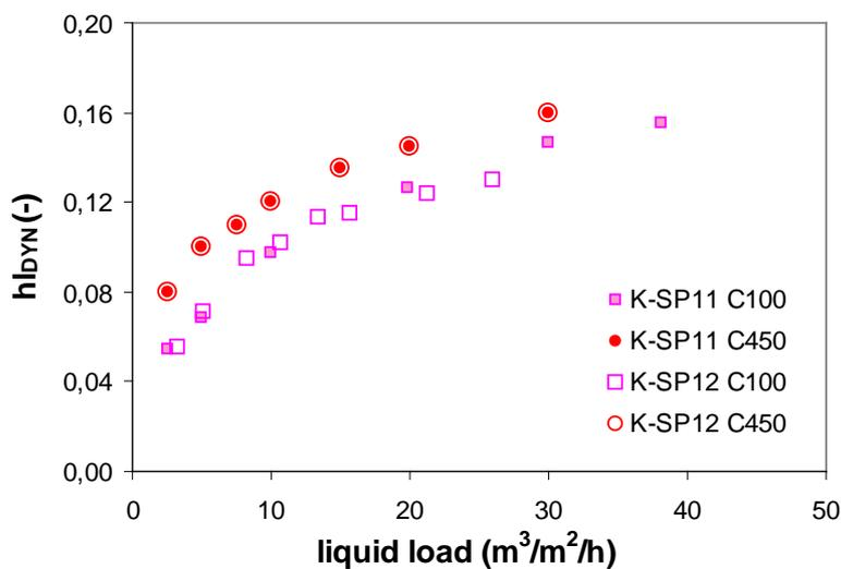
**Figure 2.** Dynamic hold-up as a function of liquid load for Katapak-SP11 (filled symbols) and Katapak-SP12 (empty symbols). Data on packings diameter of 100 mm (C100, square points) are from the present work, data on packings diameter of 450 mm (C450, circle points) are from Behrens<sup>15</sup>
