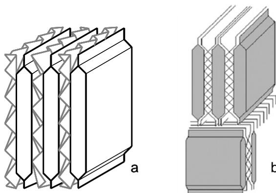
**Figure 1.** Schematic of the structure of Katapak-SP11 (a) and Katapak-SP12 (b) packings
