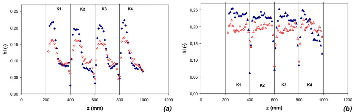
**Figure 5.** Total liquid hold-up measured on Katapak-SP11 (filled symbols) and Katapak-SP12 (empty symbols) at liquid load equals to  $4.62 \text{ m}^3/\text{m}^2/\text{h}$  (a) and  $23.1 \text{ m}^3/\text{m}^2/\text{h}$  (b)
