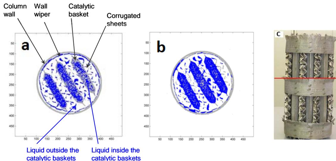
**Figure 3.** Reconstructed image of a cross section of Katapak-SP12 situated at a height of  $z=490$  mm, irrigated by a liquid load of  $4.62 \text{ m}^3/\text{m}^2/\text{h}$  (a) and  $12.7 \text{ m}^3/\text{m}^2/\text{h}$  (b), and with no gas flowrate. In (c) the horizontal line shows the position of the cross-section with respect to the packing element height
