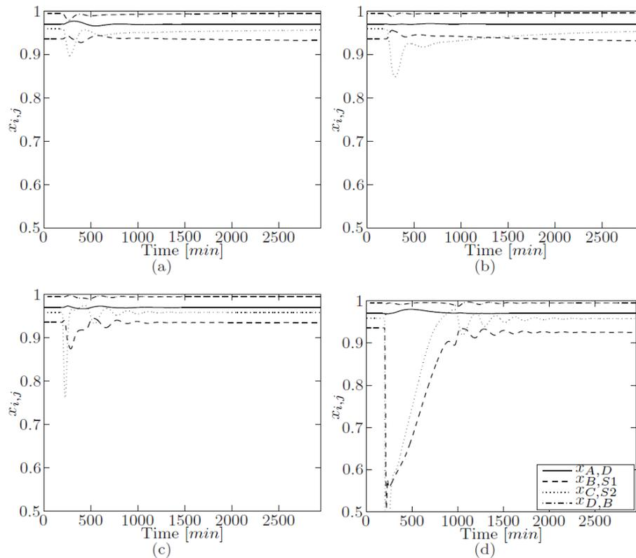
**Figure 4.** Kaibel column with 4 temperature loops closed: Disturbance responses (a)  $F + 10\%$ , (b)  $z_{B,F} + 20\%$ , (c)  $R_V + 10\%$  and (d)  $R_V + 50\%$
