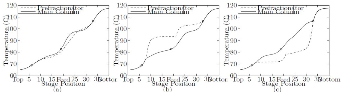
**Figure 2.** Kaibel column with 3 temperature loops closed: Column temperature profiles. (a) Nominal profile, (b)  $R_L = 0.50R_{L,opt}$ , (c)  $R_L = 1.50R_{L,opt}$ . Controlled temperatures are encircled.
