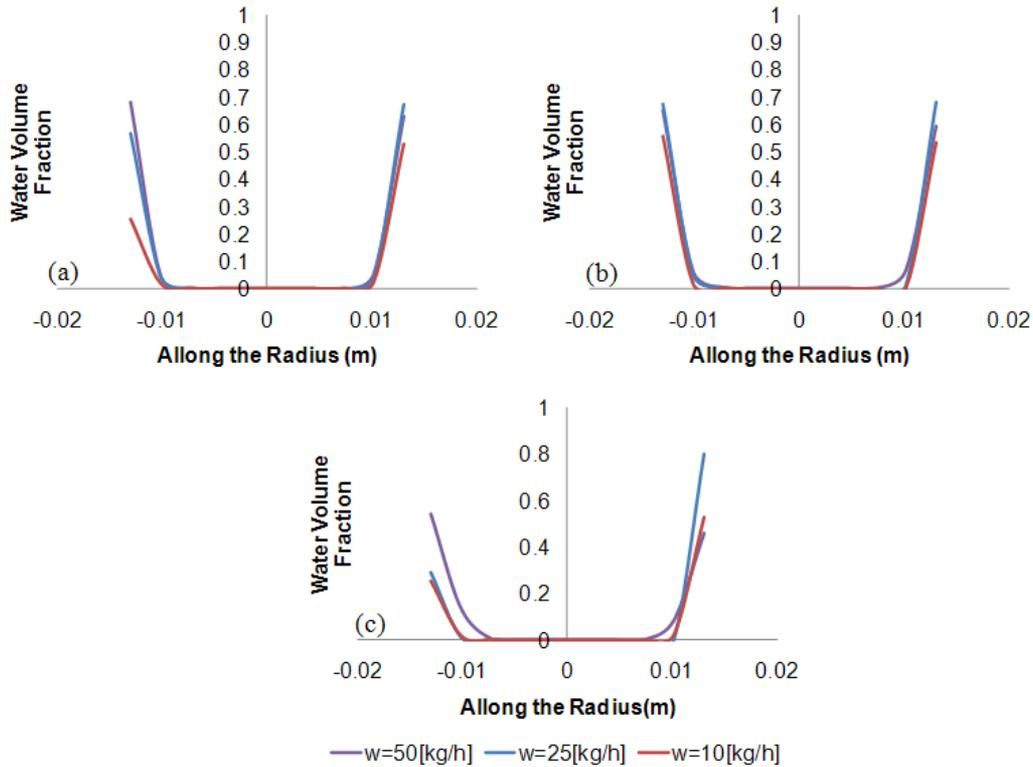
**Figure 3.** Profiles of Volumetric Fraction of Liquid (a) 10mm (b) 65mm and (c) 165mm below the feeding cone for the mass flows of 50, 25 and 10 (kg/h) with hybrid mesh.
