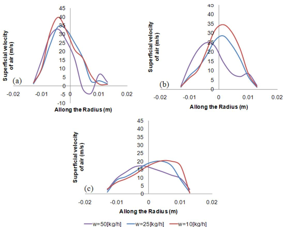
**Figure 4.** Profiles of Air Superficial Velocity (a) 10 mm (b) 65 mm and (c) 165 mm below the feeding cone for the mass flows of 50, 25 and 10 (kg/h) with hybrid mesh.
