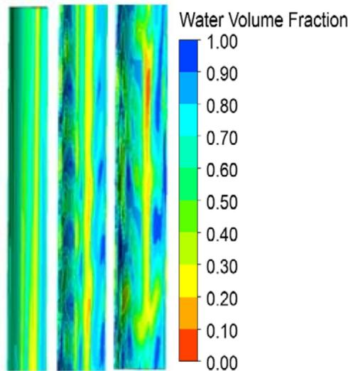
**Figure 5.** Profile of the volumetric fraction of liquid on the walls of the distillation tube with 50 (kg/h).
