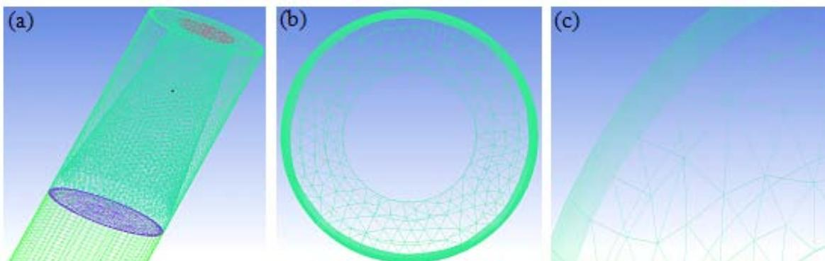
Figure 2. Hybrid mesh (a) cone (b) top view (c) mesh detail.
