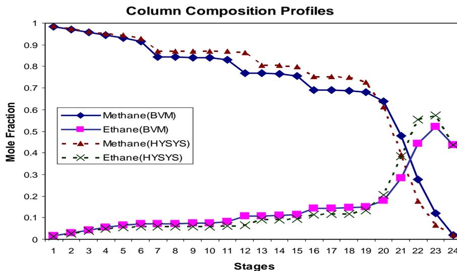
**Figure 3.** Composition profiles for key components: new model (BVM) vs. HYSYS
