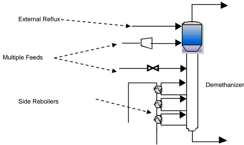
Figure 1. A typical demethanizer column
