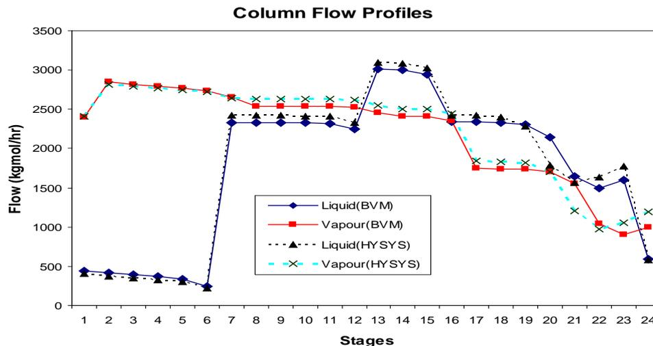
Figure 4. Molar flow profiles: new model (BVM) vs. HYSYS
