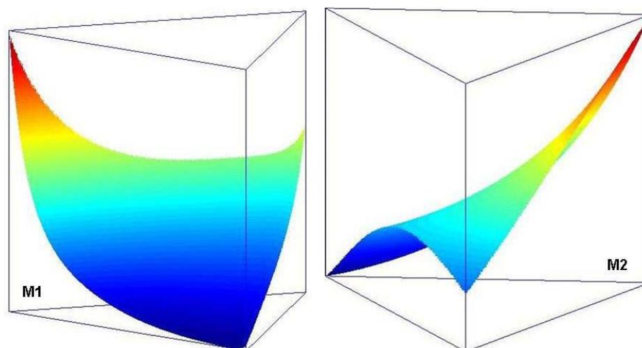
Figure 2. Boiling temperature surfaces for mixtures M1 and M2
