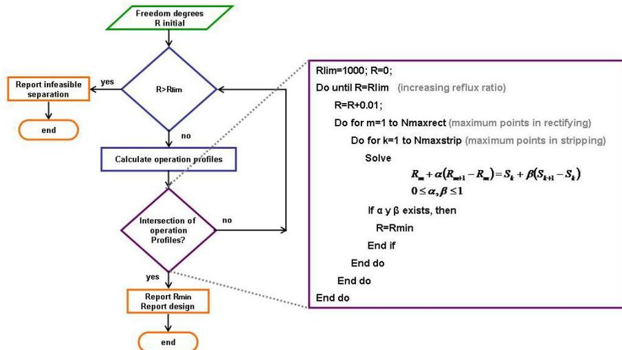
Figure 1. Algorithm and pseudo code to calculate the minimum reflux ratio
