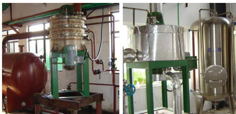
Figure 7 Onsite pictures of recovery of methanol (left) and ethanol (right) by RZB in the industrial continuous distillations
