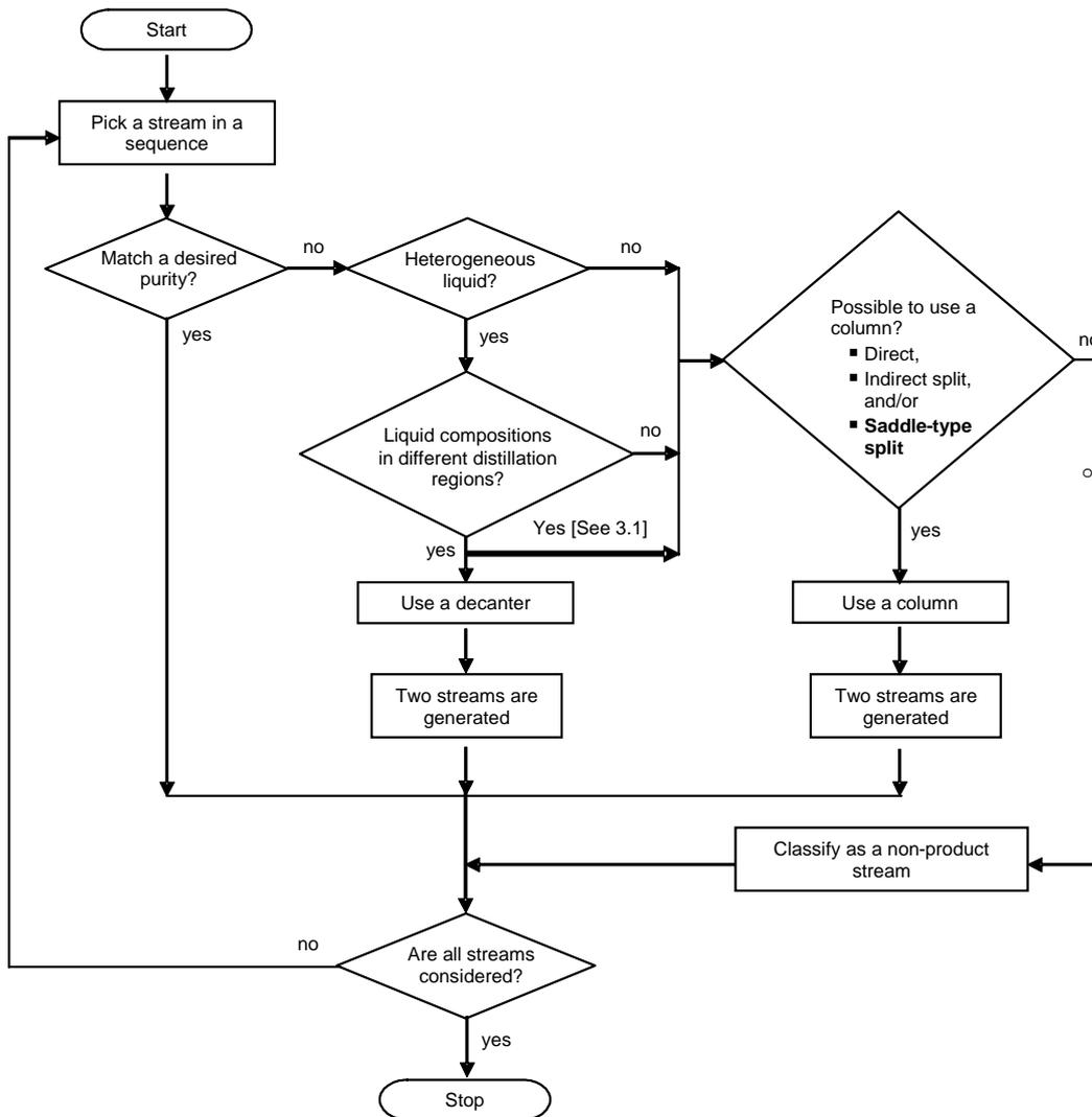
**Figure 1.** Existing algorithm<sup>3,4</sup> extended to include double-feed column and use of heterogeneous column feed (where equilibrium liquid compositions are in different distillation regions)<sup>6</sup>.
