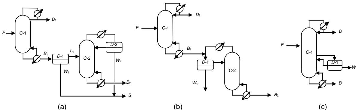
**Figure 2.** Two columns with two decanters carrying out similar separations can be merged to give a column with an intermediate decanter<sup>6</sup>.
