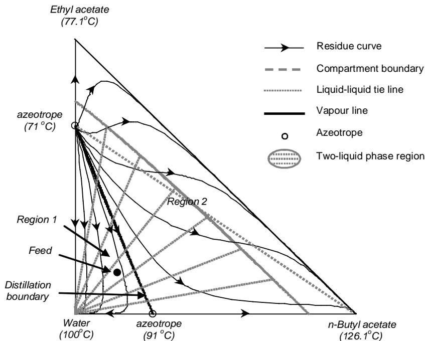
Figure 3. Residue curve map for n-butyl acetate–ethyl acetate–water mixture at 1 atm<sup>6</sup>.
