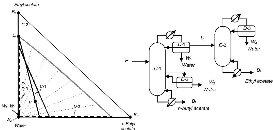
Figure 7. Option 4: Sequence evolved from Option 3, including column with intermediate decanter<sup>6</sup>.
