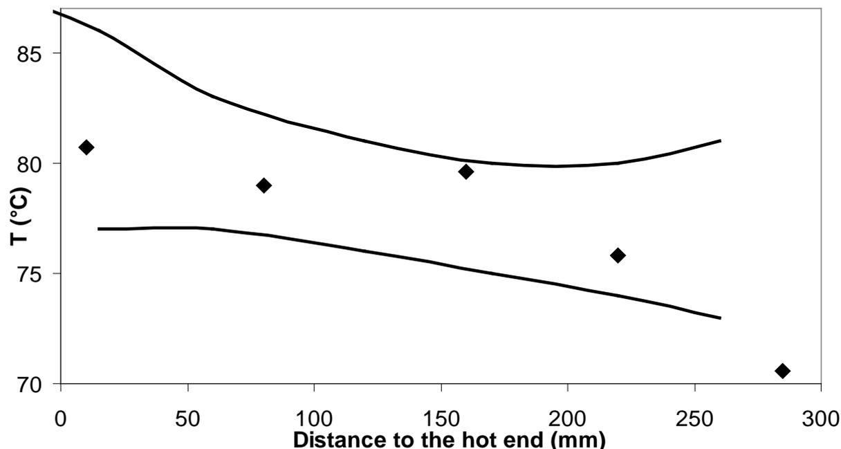
**Figure 3.** n-Hexane + Cyclohexane distillation with total reflux; reboiler section is at the left; ◆ represents the temperature inside distillation packing, solid line represents temperature profile of the aluminum plates.
