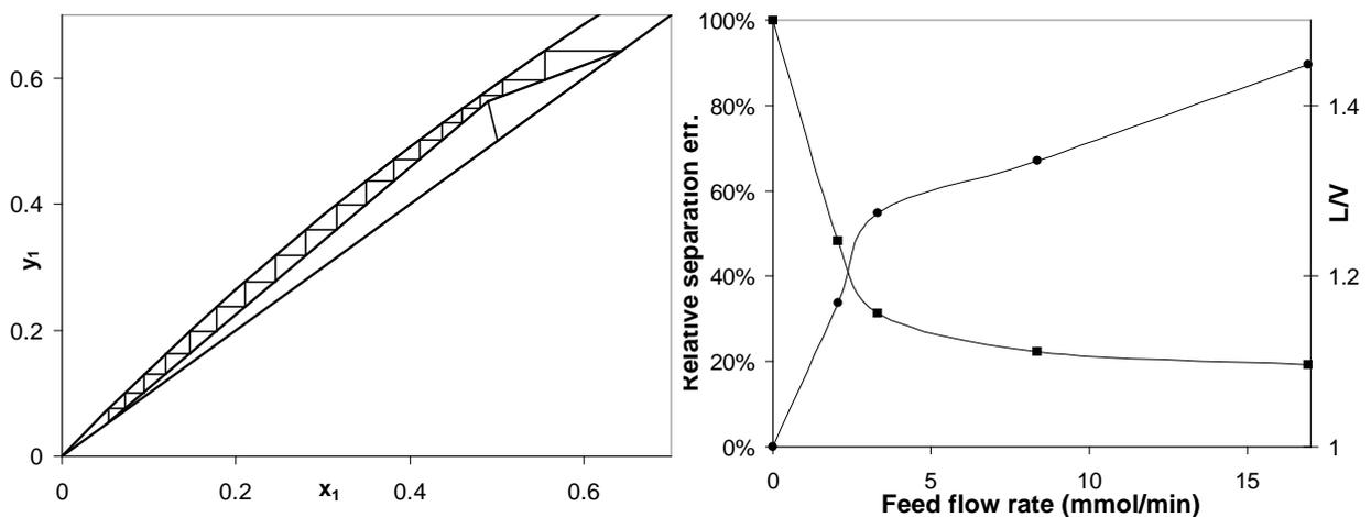
**Figure 5 (a)** McCabe-Thiele diagram for the experiment with feed flow rate of 0.25 ml/min of n-Hexane(1) + Cyclohexane **(b)** Results of the continuous flow experiments as a function of feed flow rate in mmol/min; ■ presents the relative separation efficiency compared to distillation with total reflux; ● marks the slope of the stripping line (L/V ratio)
