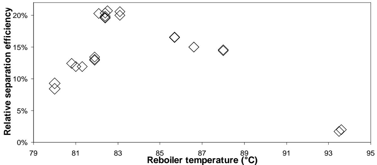
**Figure 4.** Separation efficiency with a feed flow rate of 2 ml/min of n-Hexane + Cyclohexane expressed as a fraction relative to separation with total reflux at various reboiler temperatures.
