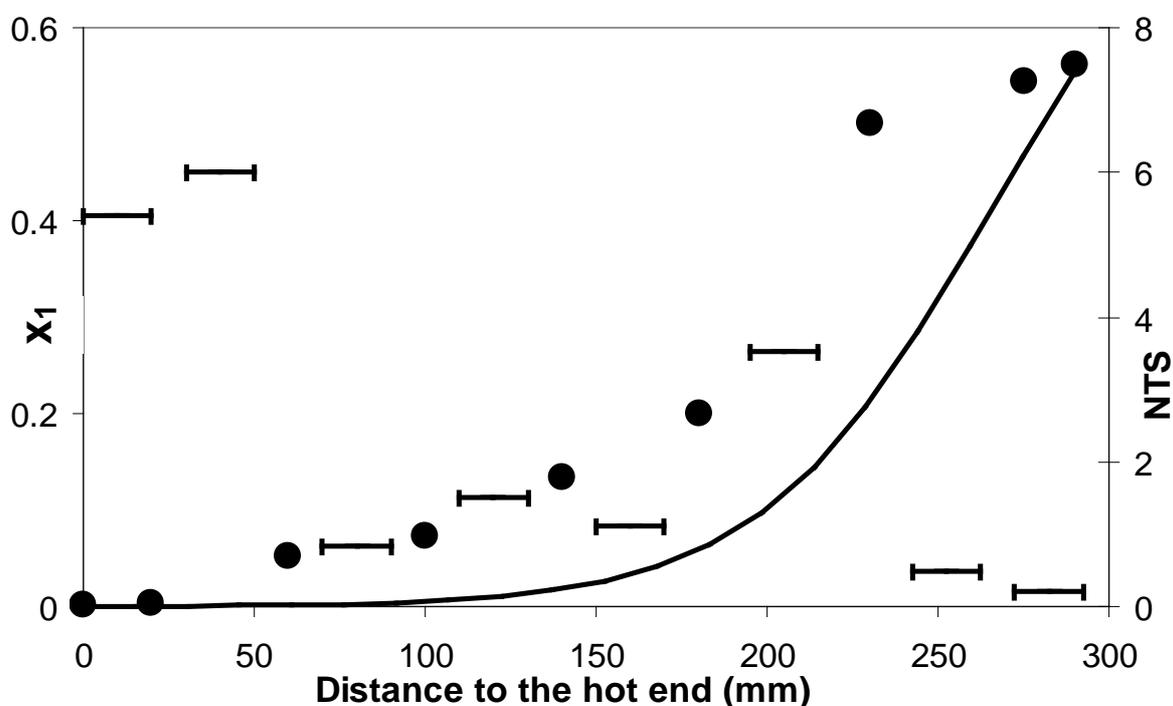
**Figure 2.** n-Hexane (1) + Cyclohexane distillation with total reflux; reboiler section is at the left; ● represents measured concentration, solid line represents simulation with total reflux, ┆ represents the number of theoretical stages between adjacent measurements.
