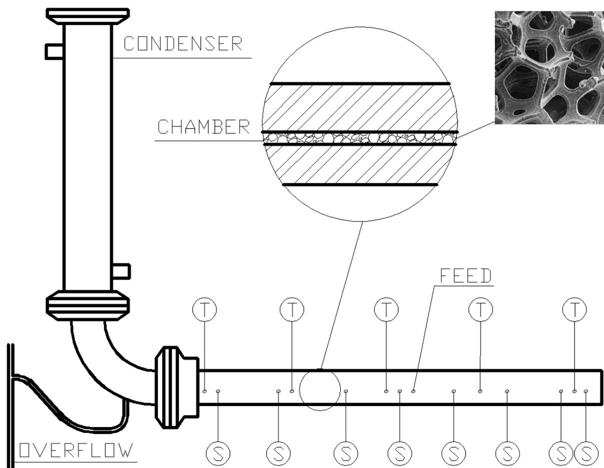
**Figure 1.** Diagram of the distillation column. S marks sampling connections and T marks temperature measurements. The right end of the column was the heated reboiler section. Aluminum plates above and below the column are not shown. Picture of the metal foam is by Recemat International<sup>7</sup>.
