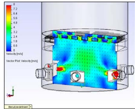
Fig. 3: CFD analysis of gas inlet
