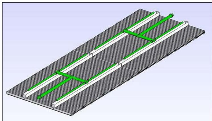
Fig. 2: Piping arrangement and liquid distributor design for a square shaped column.
