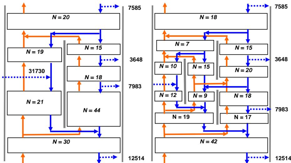
**Figure 3.** Internal configuration with stage numbers for each section and corresponding vapour and liquid flow patterns for single- and multiple-partition wall DWC, including mass flow rates (kg/h) of the feed and four product streams
