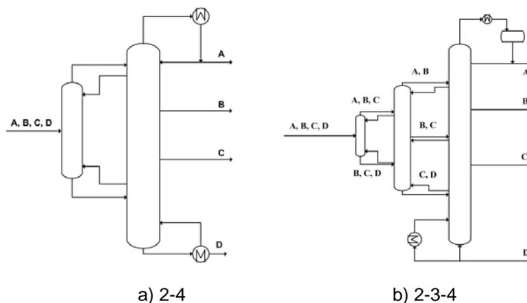
Figure 2. Simple column sequences used for rigorous simulation
