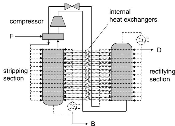
**Figure 1.** Superstructure to determine the optimal Number of trays and the position of internal heat exchangers for both column sections
