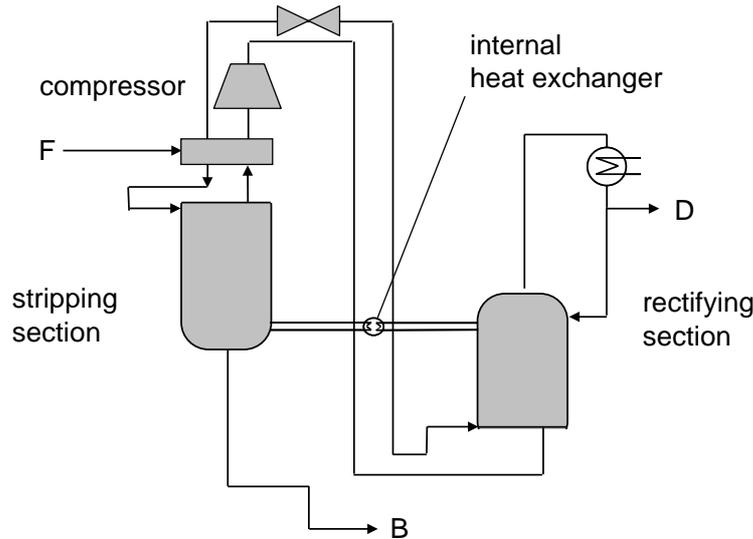
**Figure 3.** Optimal column configuration for the fluorobenzene / benzene separation
