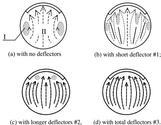
**Figure 4.** Flow patterns on trays
