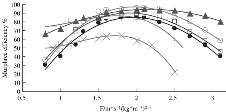
**Figure 8.** Tray efficiencies of DDV tray and traditional trays 1–DDV tray, 2–DS tray, 3–rectangle-shaped valve tray, 4–F1 tray, 5–deflected sieve tray, 6–sieve tray
