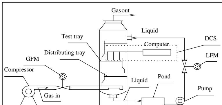
**Figure 2.** Schematic diagram of the experimental apparatus
