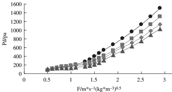
**Figure 5.** Pressure drop per dry tray at different F-factor ( $L = 15.5 \text{ m}^3 \cdot \text{h}^{-1}$ ) ◆ traditional F1 tray; ■ rectangular-shaped valve tray, ● DS tray, ▲ DDV tray
