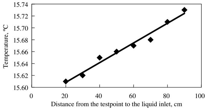
**Figure 7.** Horizontal temperature profile of the liquid layer on DDV tray
