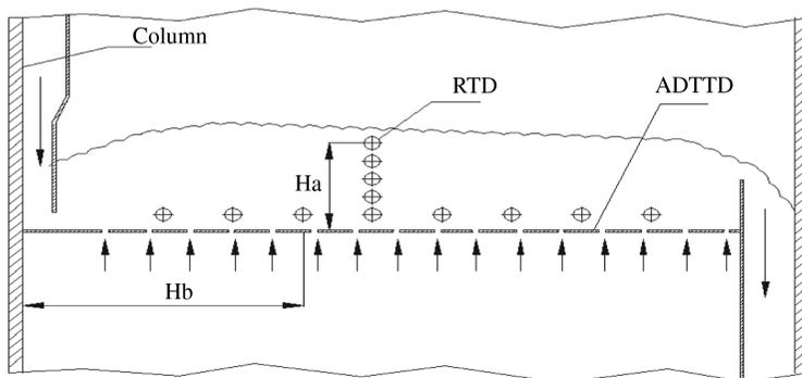
**Figure 3.** Positions of RTDs;  $H_a$ , distance from the testpoint of the RTD to the tray surface, equal to the height of the liquid layer;  $H_b$ , distance from the testpoint to the liquid inlet
