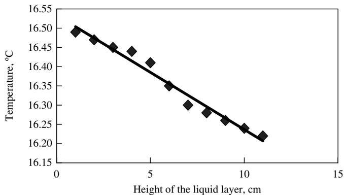
**Figure 6.** Vertical temperature profile of the liquid layer on DDV tray
