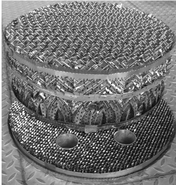
**Figure 1.** The sandwich packing of the 2. generation – combination of a Montz Pak 750T as flooded layer and a Montz Pak 250 M as de-entrainment layer (500 m diameter)
