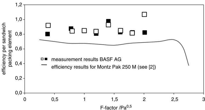
**Figure 3.** Efficiency of the sandwich packing (combination Montz Pak 750T/250M, column diameter of 500 mm) tested with methylcyclohexane/n-heptane at 1.6 bar pressure and compared with measurement results for the conventional Montz-Pak 250M tested with a mixture of cyclohexane/n-heptane at pressure of 1 bar
