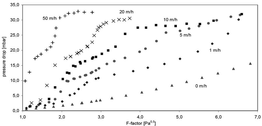
**Figure 2.** Pressure drop of the sandwich packing combination Montz Pak 750T/250M for liquid loads from 0 to 50 m/h, measured in an air/water-column with 500 mm column diameter
