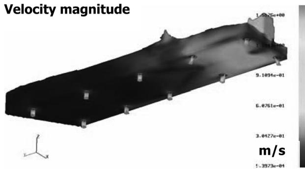
**Figure 9.** Fluid flow through the 10 orifices of the second arm after 2.05 s at minimum load
