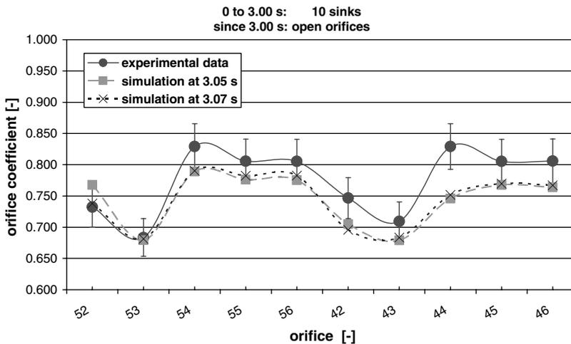
**Figure 10.** Simulated local orifice coefficients including experimental validation numbering refer to Figure 7
