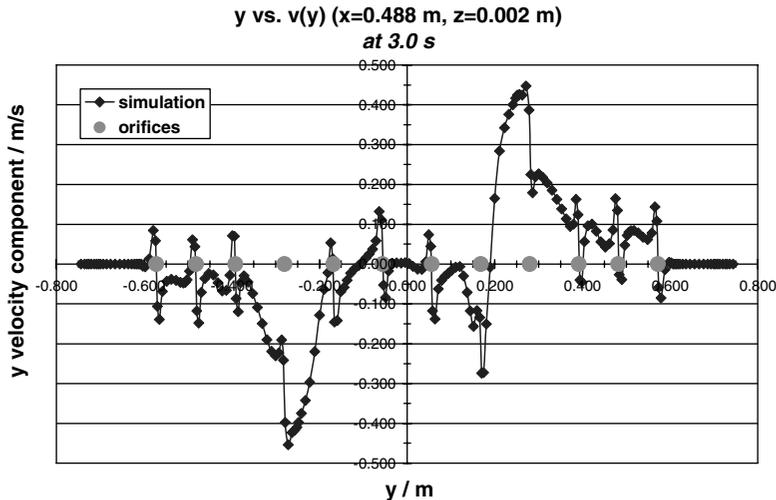
**Figure 8.** Quantitative assessment of lateral velocity acc. to Figure 7 using different grids
