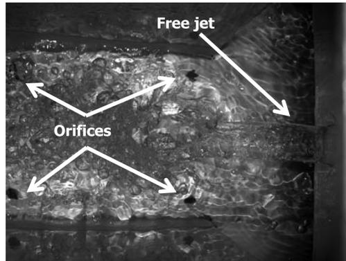
**Figure 11.** Free jet flow through lateral orifice of pre-distributor into the 2nd channel
