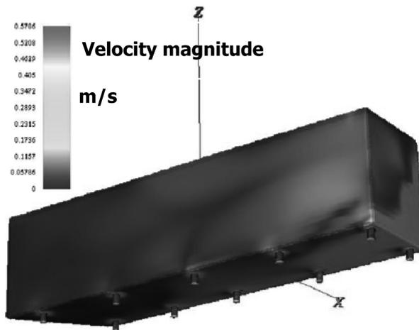
**Figure 12.** Fluid flow through the 10 orifices of the second arm after 2.05 s at nominal load
