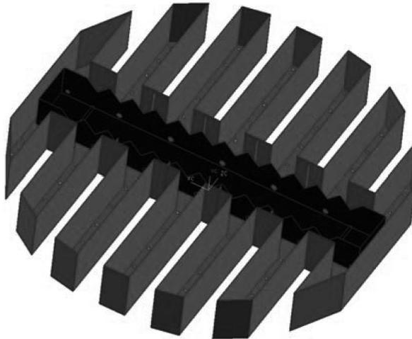
**Figure 5.** Channel distributor including pre-distributor
