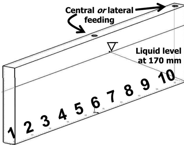
Figure 2. Single channel with central or lateral feeding (26 × 600 × 230 mm)
