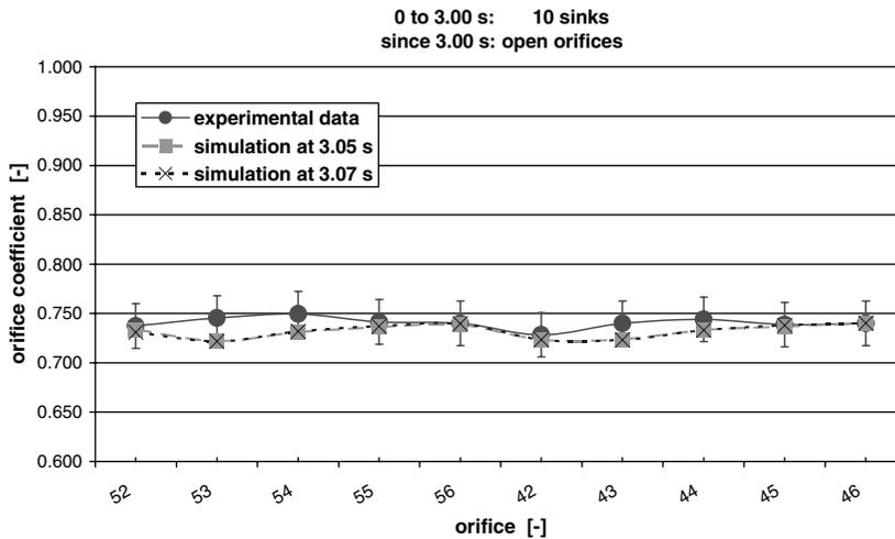
**Figure 13.** Simulated local orifice coefficients including experimental validation numbering refer to Figure 7
