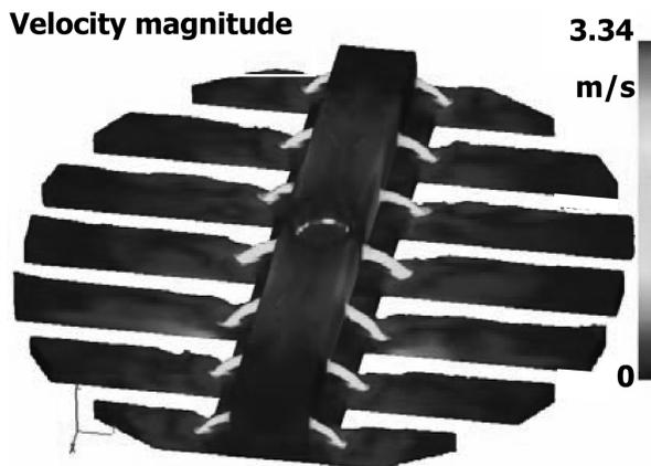
**Figure 6.** Fluid flow on a channel distributor including pre-distributor
