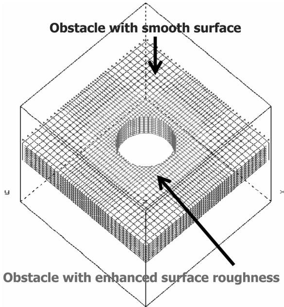
Figure 1. Ring around the orifice possessing surface roughness
