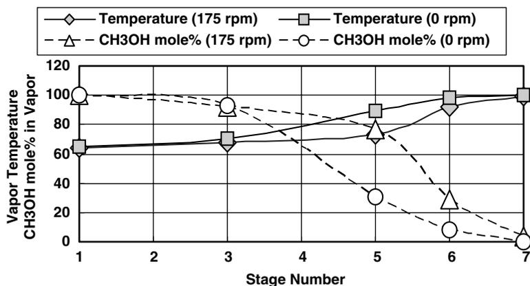
**Figure 7.** Distribution of vapor temperature and methanol concentration in vapor in the test column operated under total reflux condition
