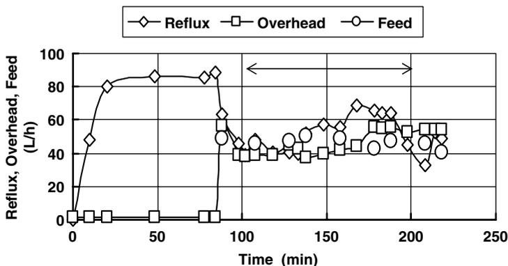
**Figure 8.** Temporal variation of reflux, overhead product and feed rates (Operation Record)
