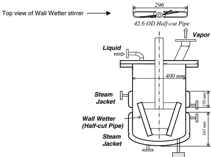
Figure 2. Wall Wetter evaporator for reboiler
