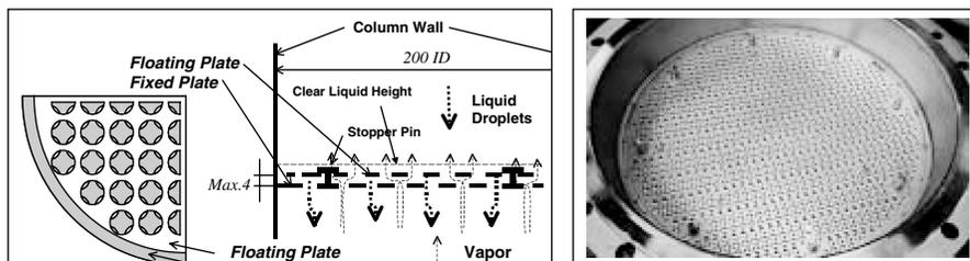
**Figure 3.** Dual flow tray “Lift Tray” and its photograph of a large tray for a 900 mm ID column
