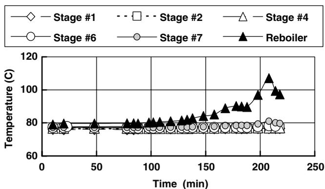
**Figure 9.** Vapor temperature trajectory of each stage in the quasi-steady operation period
