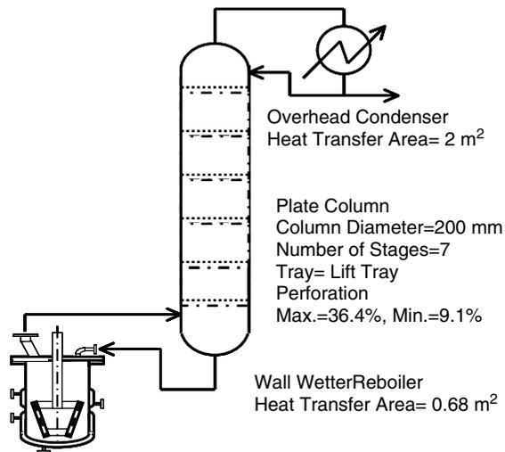
Figure 1. Experimental setup for batch distillation
