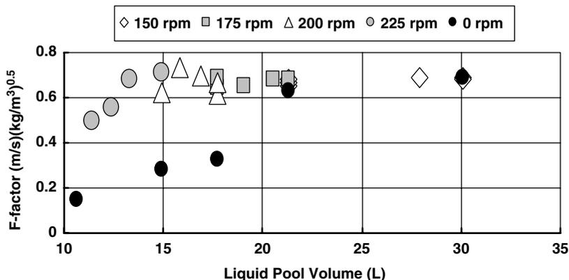
**Figure 5.** Effect of Wall Wetter rotation on the relation of F-factor with liquid volume
