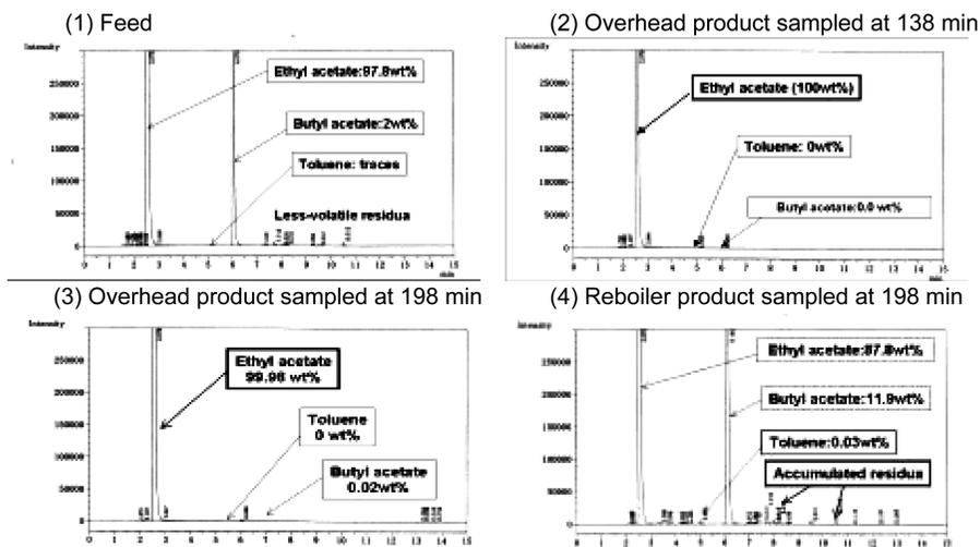
**Figure 10.** Gas chromatograms of composition of overhead product and reboiler solution in the quasi-steady operation term with the feed composition
