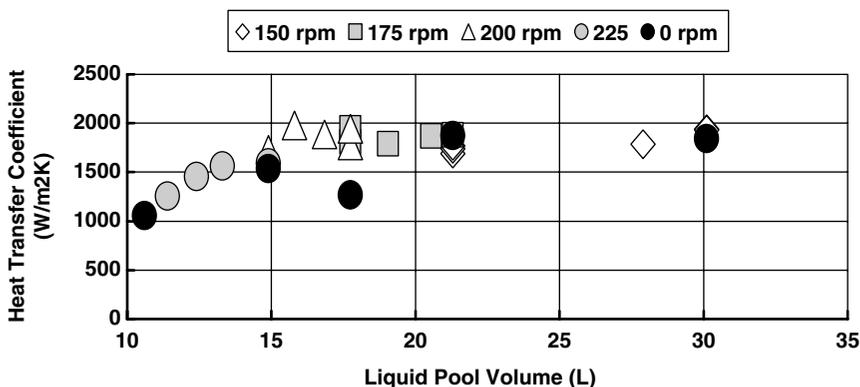
**Figure 6.** Heat transfer coefficient on the inner wall of the reboiler
