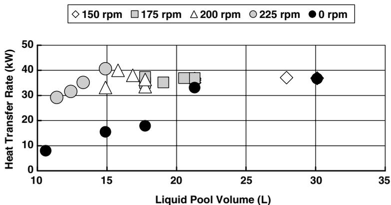
**Figure 4.** Variation of heat transfer rate with liquid pool volume
