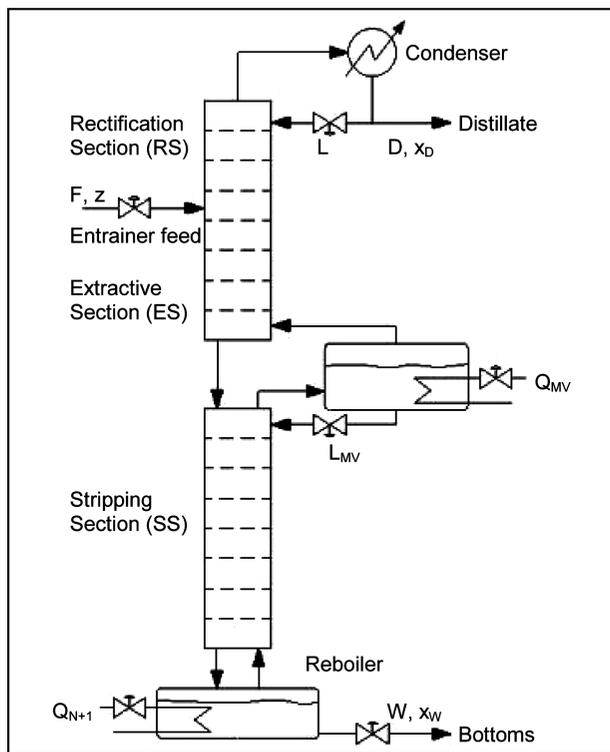
**Figure 3.** Extractive MVC (liquid bypass version)
