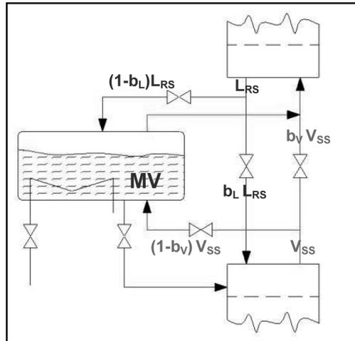
**Figure 2.** Middle section of a general MVC ( $b_L \geq 0$ ,  $b_V \geq 0$ )
