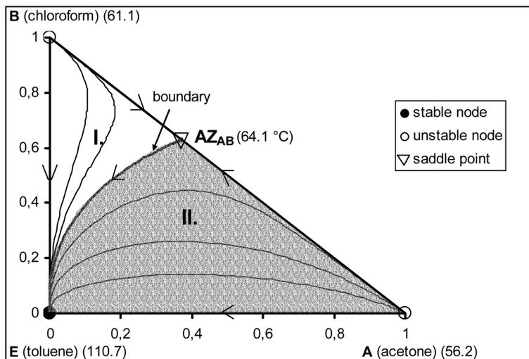
**Figure 4.** The residue curve map and batch distillation regions
