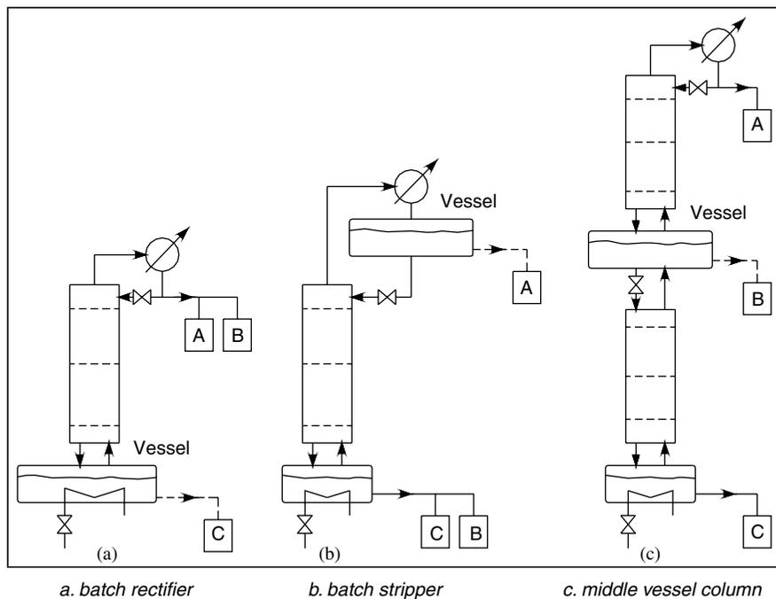
**Figure 1.** Batch distillation column configurations
