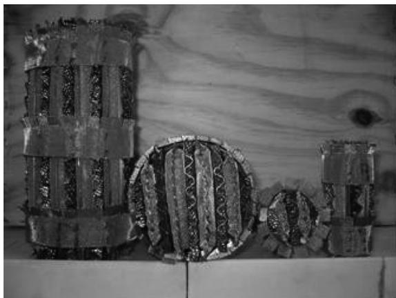
**Figure 1.** Katapak<sup>®</sup>-SP 11 elements with nominal diameters of 100 and 50 mm
