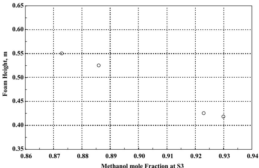
**Figure 5.** Effect of methanol concentration on foam height
