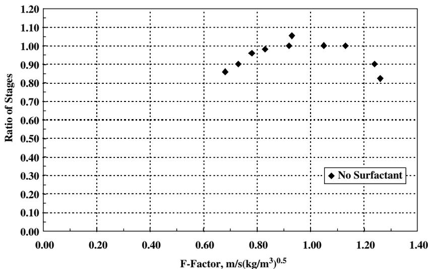
Figure 2. Measured efficiency (without surfactant)
