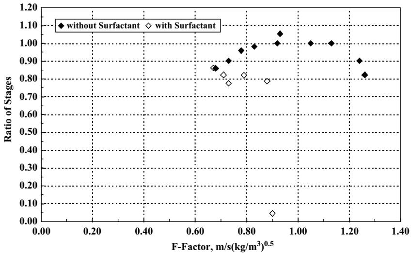
Figure 6. Effect of foaming on efficiency
