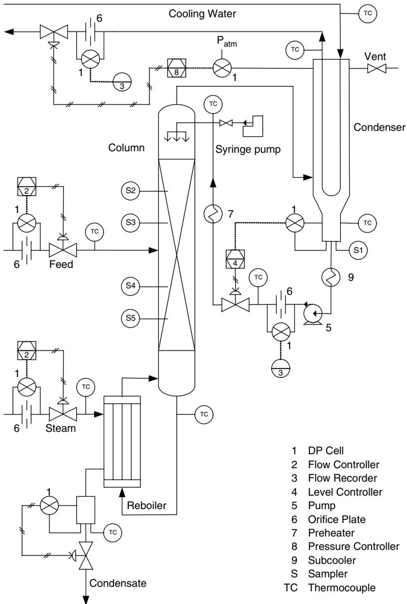
**Figure 1.** Schematic diagram of experimental setup
