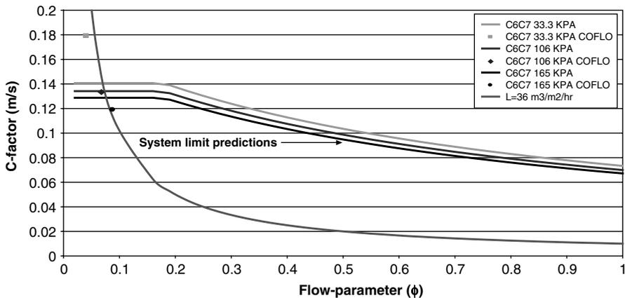
**Figure 1.** COFLO [9] flood points at different pressures compared with the system limit correlation
