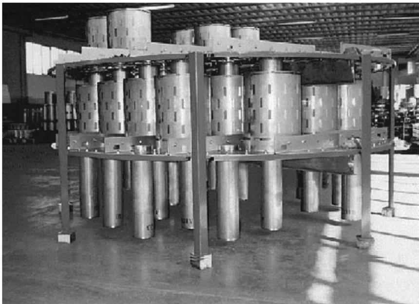
**Figure 2.** Photograph of an ULTRA-FRAC<sup>®</sup> tray assembly
